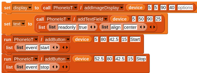
Fig. 5. Blocks used to set up the PhoneIoT device display for the GPS tracker.
